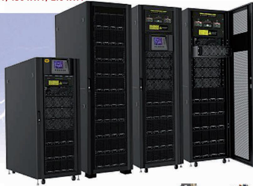
ORVALDI Power series is a modular power supply that is characterized by high performance and overload capacity. The power of a single module is 30kW, and the maximum power of one cabinet is 210kW. Modular construction allows for live replacement and rapid power expansion.
